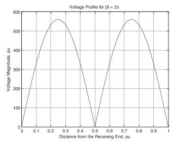
**Fig. 2.** Voltage profile with n = 2.
