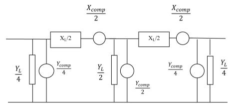
Fig. 6. Equivalent circuit of transmission line with beta compensation.
