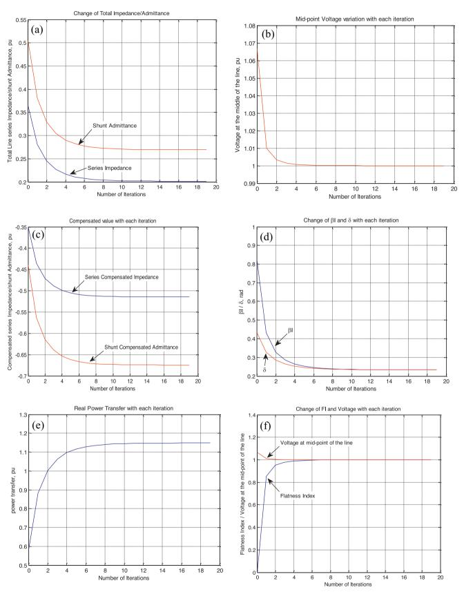
**Fig. 9.** (a) Total line parameters variation. (b) Mid-point voltage variation. (c) Compensator variation. (d) δ and βl variation. (e) Variation of real power transfer. (f) Flatness Index variation.
