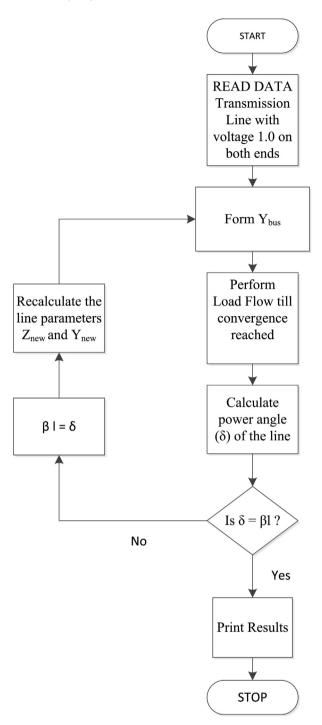
Fig. 5. Flow chart of the beta compensation method.
