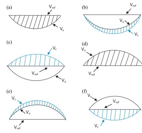
**Fig. 7.** (a) Voltage profile of sag case with proper compensation. (b) Voltage profile of sag case with improper compensation. (c) Voltage profile of sag case with over compensation. (d) Voltage profile of hump case with proper compensation. (e) Voltage profile of hump case with improper compensation. (f) Voltage profile of hump case with over compensation.
