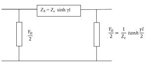
Fig. 1. Long line equivalent circuit.
