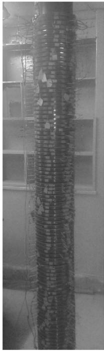
**Fig. 1.** Analog and simulated model of 3 MVA, 33/11 kV, 3-phase power transformer. (Courtesy: High voltage laboratory, Jadavpur University, India) [29].
