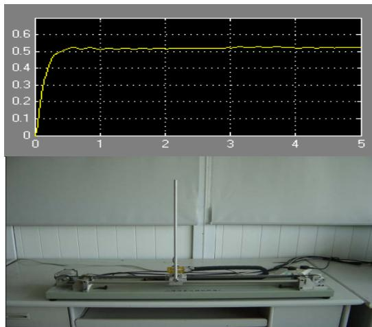
Fig.9 The experimental result of the inverted pendulum
