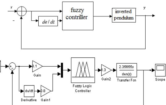
Fig.6. Simulation structure of the inverted pendulum
