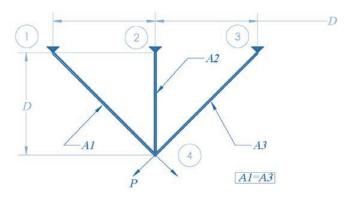
Fig. 11. Three-bar truss design problem.
