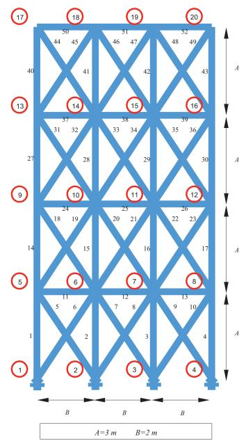
Fig. 13. Structure of a 52-bar truss.
