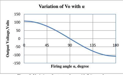
Figure 8. Variation of output voltage with firing angle
