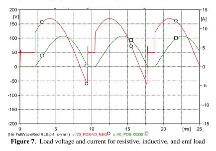
The average value of the output voltage is given below [5]-[7]:  $Vo = \frac{2Vm}{\pi} \cos \alpha \quad \dots \quad (7)$
