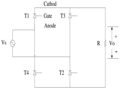
Figure 2. Single-phase full-wave bridge rectifier with R load
