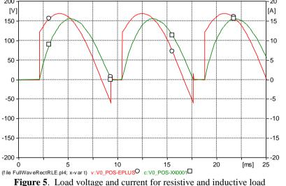
It can be seen from Fig 5 that the output current is zero when  $\omega t = \alpha$  and  $\omega t = \beta$ . If the inductance value is large, output current becomes continuous and comparatively ripple free. The average output voltage Vo can be given as below [5]-[7]:  $Vo = \frac{2Vm}{\pi} \cos \alpha$  ------(5)
