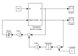
Fig.10: Simulink block diagram representing close loop Scheme of Boost converter using cascaded control
