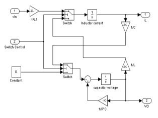
Fig. 6: Open-loop of Buck-Boost DC-DC Converters
