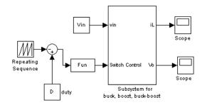
Fig. 9(a): Subsystem for Buck, Boost and Buck-Boost converters
