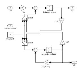
Fig. 4: Open-loop modeling of Boost DC-DC converters
