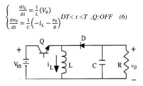
Fig. 5: DC-DC Buck-Boost Converter
