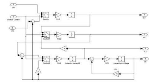
Fig. 8 Open-loop modeling of Cuk DC-DC converters
