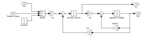
Fig 2: Open-loop modeling of Buck DC-DC converters
