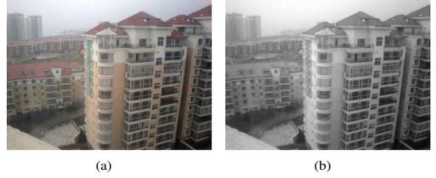
Fig. 1. Conversion from color image to the gray image in the HSV space. (a) input color image, (b) converted gray level image in the V-channel.
